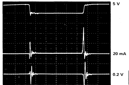
f) SN74AS00 load: C_L = 50 \text{ pF}
