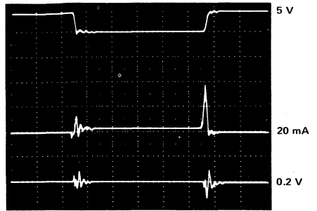
b) SN74S00 load: C_L = 50 \text{ pF}
