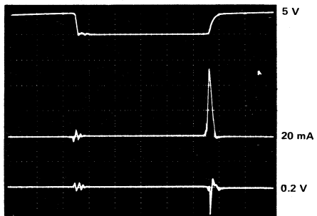
l) SN74ALS1000A load: C_L = 50 \text{ pF}
