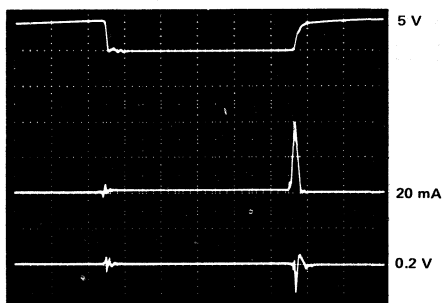
j) SN74ALS00A load: C_L = 50 \text{ pF}
